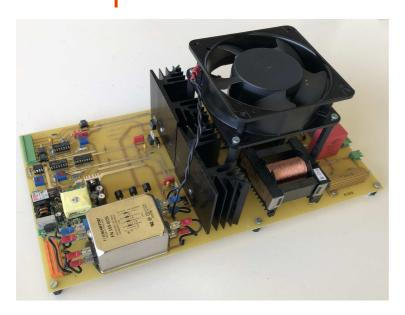
The ALM05 high frequency switching current generator is intended to load the capacitor bank of optically pumped lasers ML05 in a reproducible and adjustable manner.
